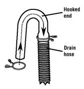
**STEP 3.** Put hooked end of drain hose into laundry tub or standpipe. Check for proper length of drain hose. Rotate hook to eliminate kinks.
